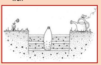
4. Using a candle and a needle (stick it in a cork to prevent burning your fingers) burn 16 holes in the side of a 2 litre plastic bottle which has a lid. The holes should be arranged in 4 vertical rows as shown on the left.
